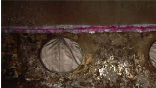
Dye penetrate reveals extensive corrosion in weld seams of spray tower
